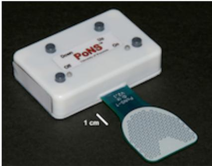
The Portable Neuromodulation Stimulator (PoNS) device passes electrical stimulation into the brain via the tongue.
